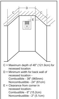
Figure 7 - Minimum Clearances for Termination Cap
